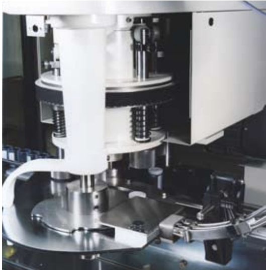
Close up of a twin turret press on capper, shown lidding 35 mm film tubs
