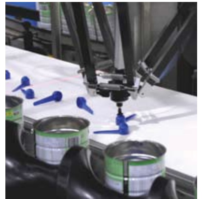
Robot Scoop placing system
