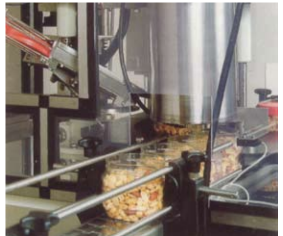
Single spindle with nitrogen flushing unit prior to cap application
